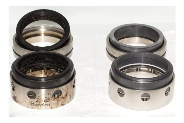
Environmentally friendly solutions in the business of mechanical repairs to pumps and compressors are readily available, and most often result in cost savings to the end user of such equipment. Reconditioning of worn components eliminates the expensive waste created by parts replacement and, as a side benefit, allows for improvements that lead to longer life cycles.
